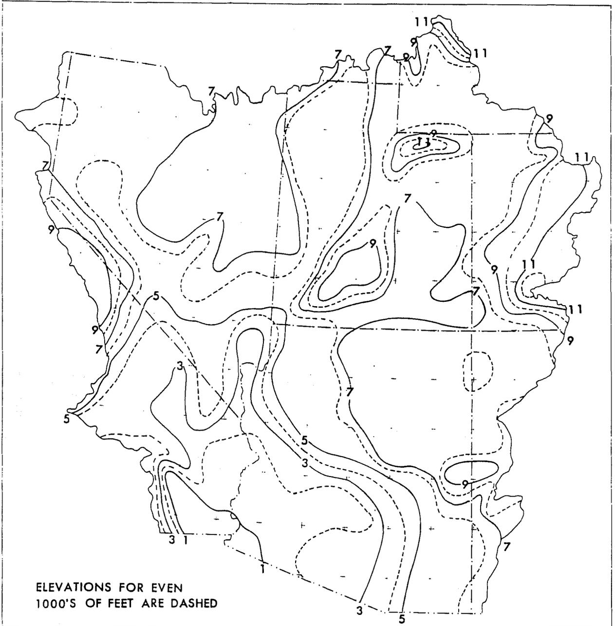
Figure 2.17.--Effective barrier and elevation heights (1000's of feet) for Southwestern States.
